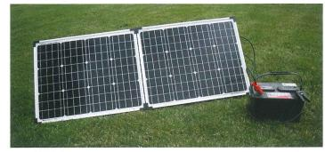
**Batteries** are used to store the power your panels produce. Battery capacity is determined by multiplying the Voltage (V) by the Amps (Ah) to get the Watt-hours (Wh). Example: a 12V 100Ah battery can store 1,200Wh of power. Batteries come in a wide range of sizes and chemistries. Your optimal battery choice will depend on what you're using them for, your budget and the conditions of use.
